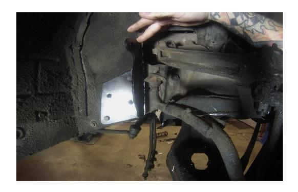
6. Now, jack the control arm up into slammed height. Mark the lower arm for lower shock mount and drill. The measurement will vary per car.
