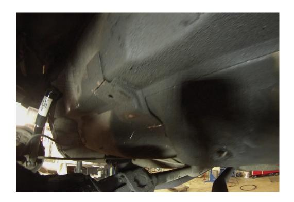
12. Next, test-fit the crossmember. It will only fit one way and sometimes tricky to get in. The lower outside hole should line up for reference. Make sure it's as high as it can go. Then mark and drill all six holes. We make a template of the side of the crossmember and use it to drill from the inside of the wheel well.
